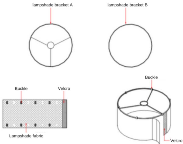
Roll the Lampshade fabric along the bracket and stick with Velcro
